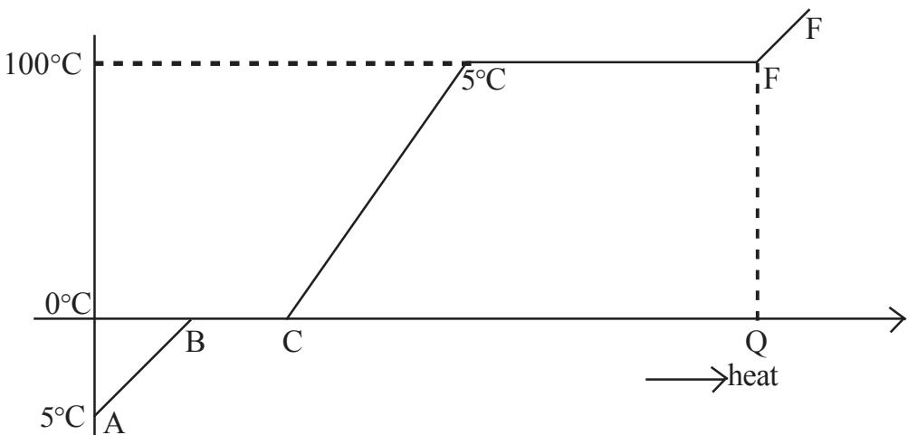
The graph given above shows that an ice of 1kg. at  $-5^{\circ}\text{C}$  is heated till it vaporises completely.
