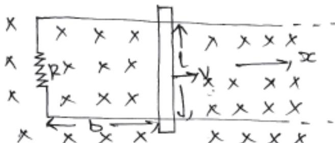
Uniform magnetic field 'B' is acting vertically downwards as shown in figure. A circuit of unthreaded wire with resistance  $R$  is kept in the magnetic field. A conductor of length  $l$  is placed on the circuit and is moving in  $x$ -direction.
